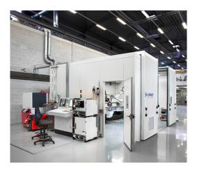
It is composed of a 6-axis robot and three different deposition heads: LMD (laser metal deposition), WLAM (wire laser additive manufacturing) and WAAM (wire arc additive manufacturing). Thus, the feed material can be either a wire or powder and the material is molten either by a laser or electrical arc. This equipment is meant to build large and very large parts, there are 3 external manipulators:
