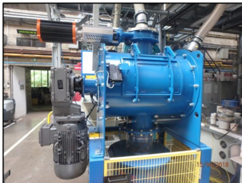
Ploughshare horizontal mixer (nominal capacity of 200 L)
