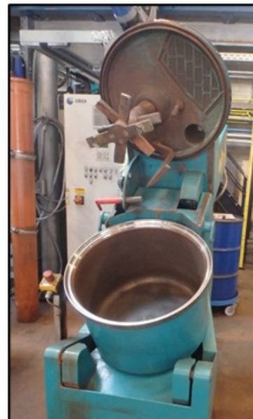
Eirich intensive mixers (nominal capacities of 5, 40 and 400 L)
