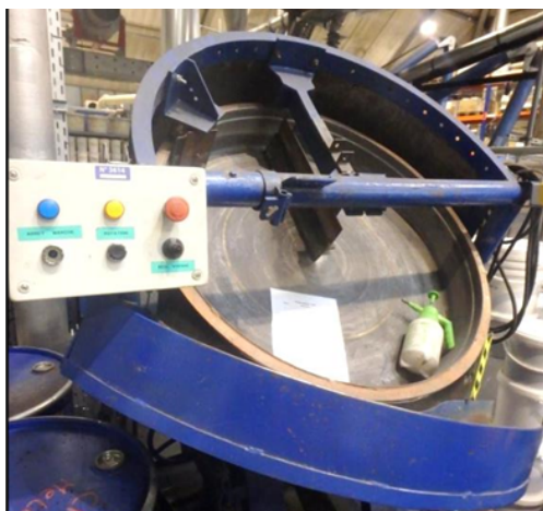
Pelletizing disks (diameter: 400, 1000, 1400 mm)
