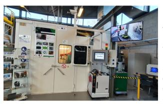
CRM Group is equipped with a 6-axis robotized thermal spray system on which different coating technologies can be adapted depending on the type of coating materials that is needed. Several technologies are available: High Velocity Oxy Fuel (HVOF), atmospheric plasma spray (APS), suspension plasma spray (SPS) and arc wire spray.
