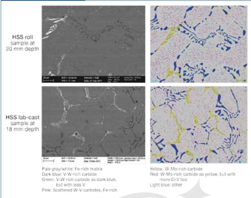
Examples phase cluster analyses by means of energy-dispersive x-ray (EDX) mappings of roll and lab-cast HSS reference samples.
