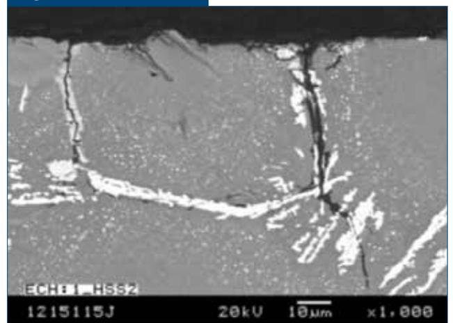
Example of fire-crazing cracks propagating preferentially along the grain boundary carbide network. Microstructure observed at an HSS sample after use in the hot rolling simulator at Centre de Recherches Métallurgiques.
