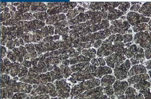
Hi-Mo HSS test block microstructure. hfw = 2,000  $\mu$ m.
