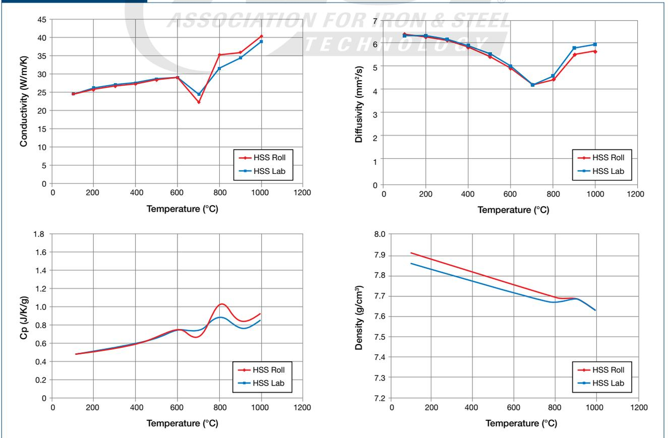
Comparison of the thermo-physical properties of roll and lab-cast HSS reference samples.
