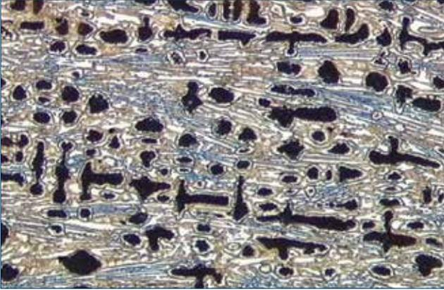
HiCr iron microstructure. hfw = 2,000  $\mu\text{m}$ .
