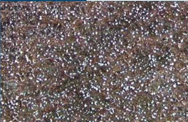
Fully heat-treated microstructure of RTB7 (HSS5). hfw = 2,000 μm.
