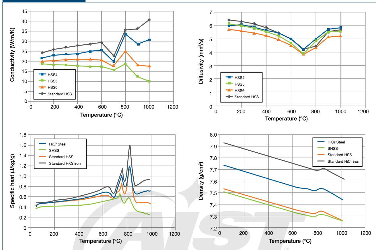
The thermophysical properties of HSS4, HSS5 and HSS6 compared to standard HSS material.
