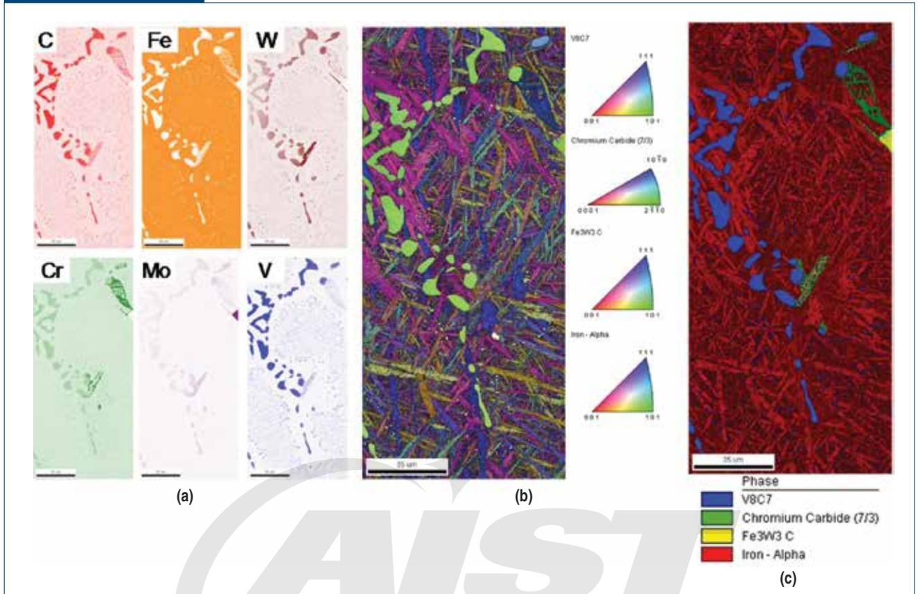
Scanning electron microscopy (SEM) + EDX + electron backscatter diffraction (EBSD) microstructure details of the reference HSS alloy (heat treated), showing the same area: in chemical composition contrast (SEM-EDX mapping) (a); in crystallographic orientation contrast (EBSD) (b); and in crystallographic phase contrast (EBSD) (c).
