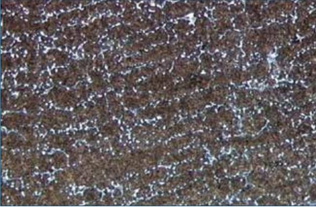
HSS6 microstructure. hfw = 2,000 μm.
