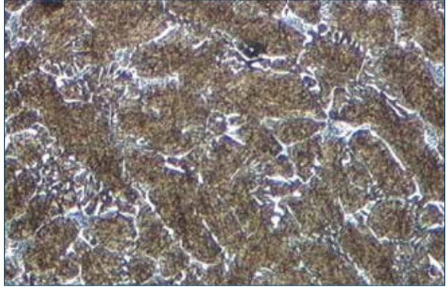
Standard HSS microstructure. hfw = 2,000  $\mu\text{m}$ .
