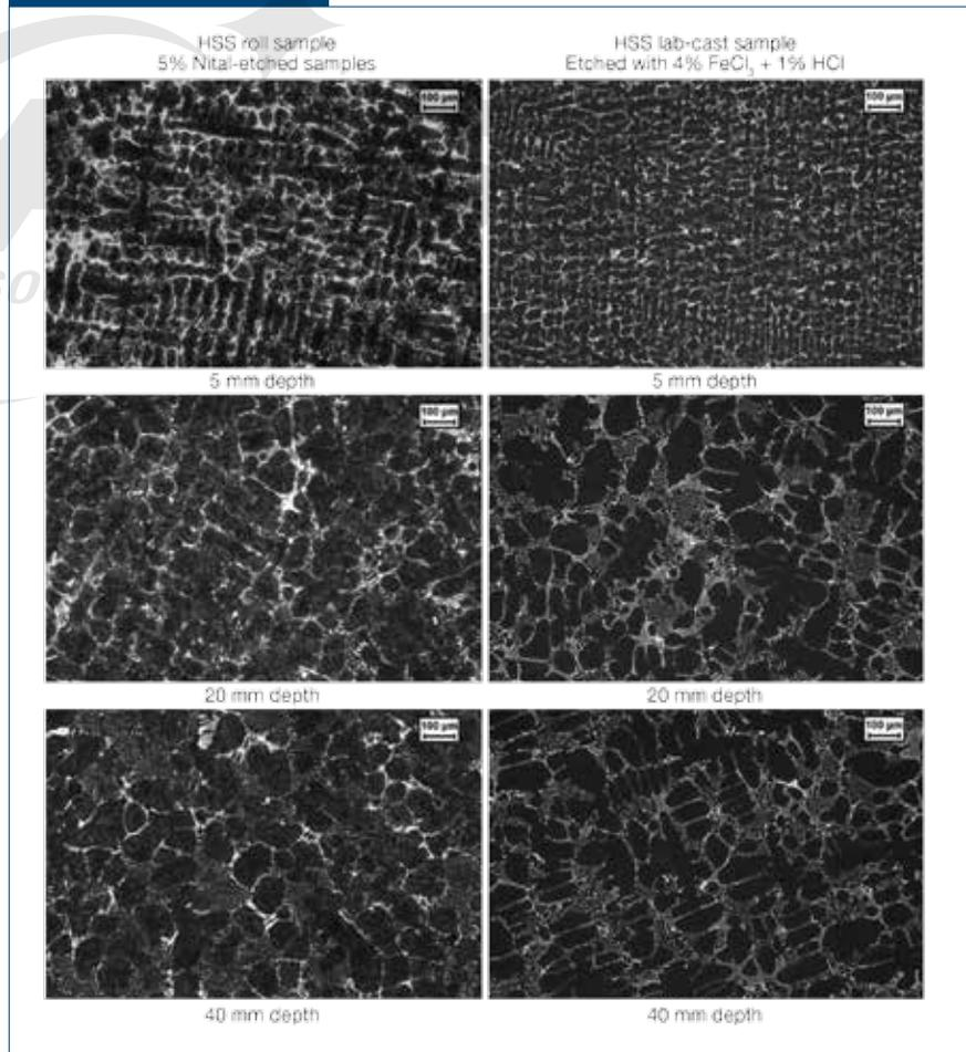
Optical microscopy images of etched roll and lab-cast HSS reference samples taken at various radial depths.
