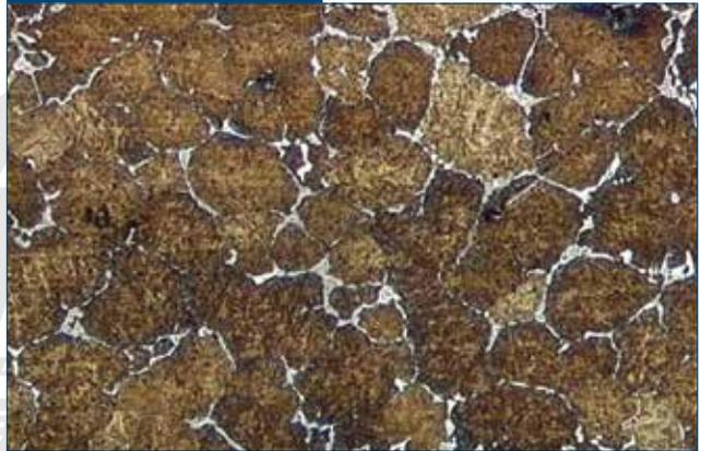
SHSS microstructure. hfw = 2,000  $\mu\text{m}$ .
