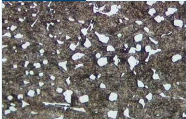
Fully heat-treated microstructure of RTB7 (HSS5). hfw = 500 μm.
