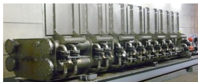
Figure 5: Tempcore design for slitting (4 lines)
