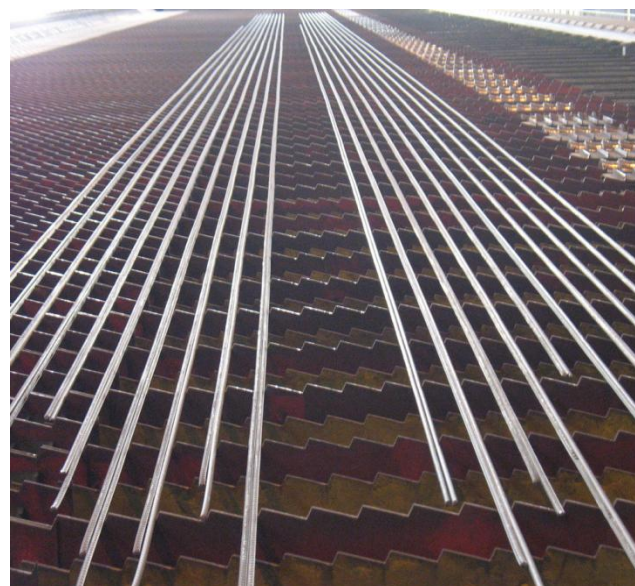
Figure 13: Straightness of slit-rebars dia 12 mm
