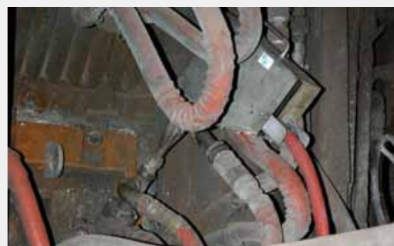
SERAFIN sensor at the back of a EAF burner
