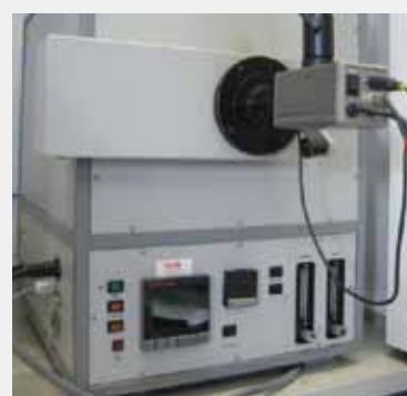
Melting unit to test sinter mixes
