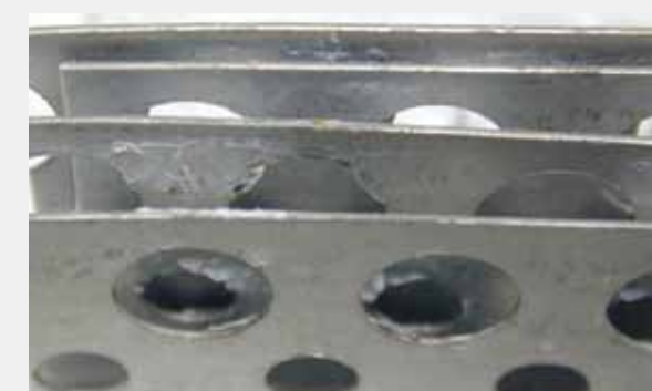
White rust problem on joining roofs
