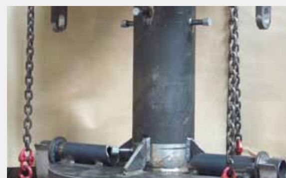
Sinter pot designed to study hot permeability
