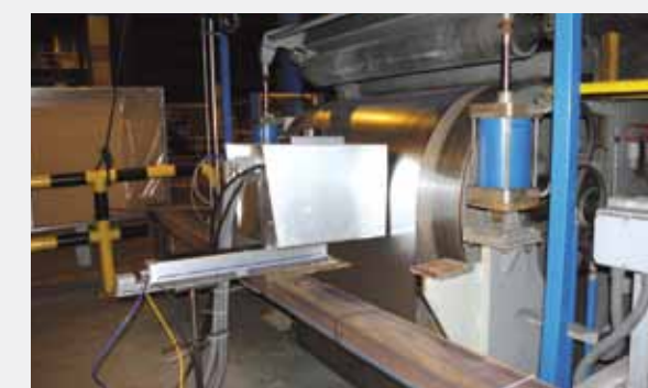
Strip waviness measurement at ArcelorMittal Avilès
