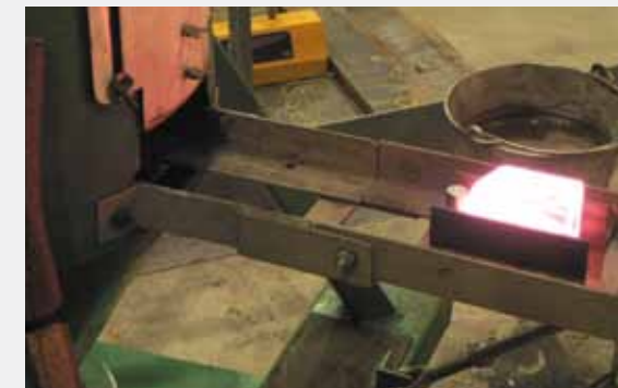
High temperature descaling by shot blasting
