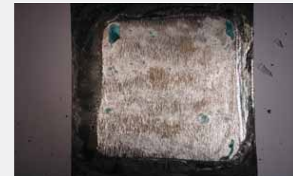
Scale prevention during heating by a glass coating
