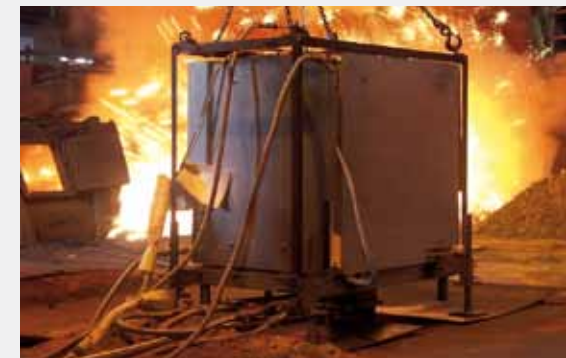
LIBS measuring unit at ArcelorMittal Ghent
