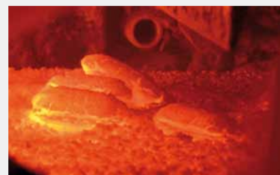
Direct reduction of self-reducing briquettes
