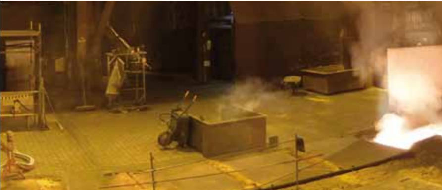
■ Continuous measurement of hot metal composition with the LIBS unit at ArcelorMittal Ghent
