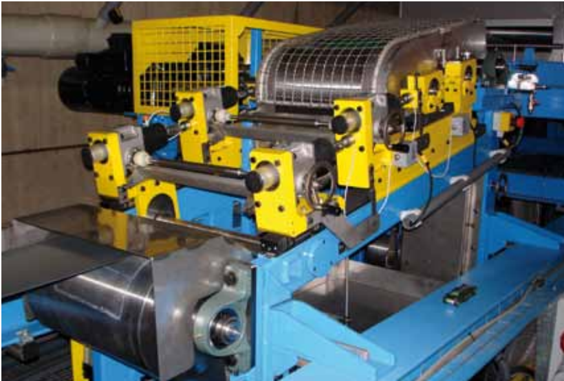
■ The new roll-coater in the CASTL line
