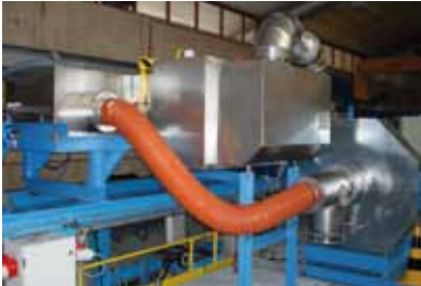
■ The new strip air-dryer in the CASTL line
