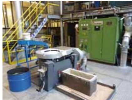
■ The new 350 kg induction furnace
