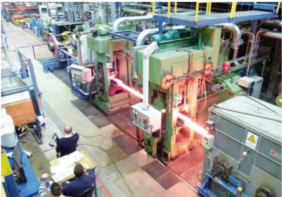
■ Continuous hot rolling trial at CRM Ghent (10 mm thick strip)
