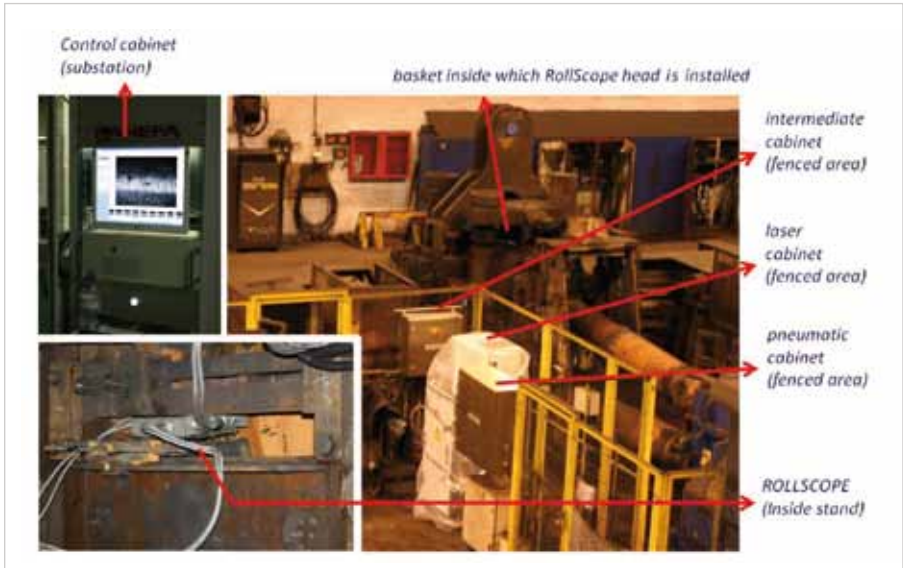
■ Industrial application of the Rollscope at Tata Steel Scunthorpe
