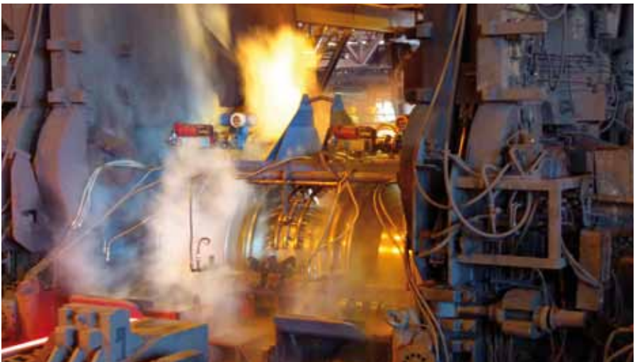
■ Industrial trial with the selective cooling system at ArcelorMittal Belval
