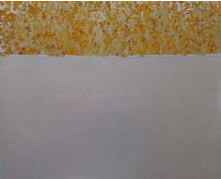
■ Bi-layers zinc-free coating after an outdoor exposure of 28 days
