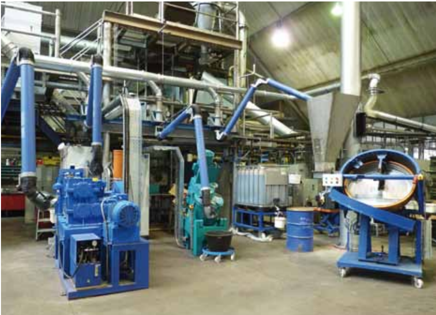
■ Preconditioning units for recycled and raw materials equipped with a flexible dust and fumes collection
