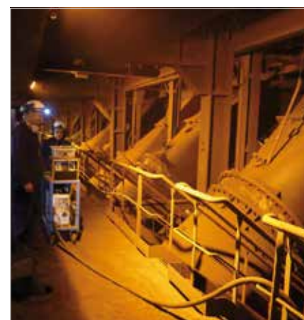
On-site measurement of gas composition and temperature in wind boxes of a sinter plant
