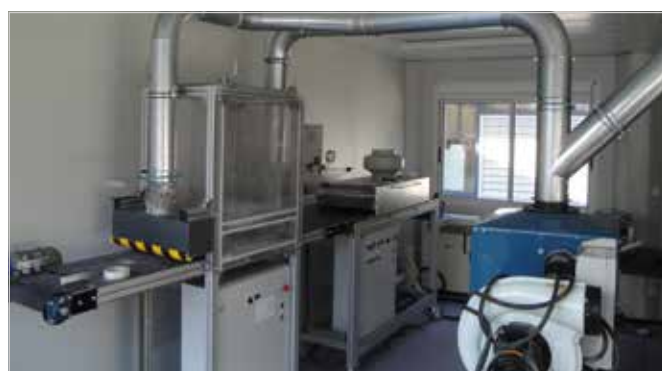
Equipment for the powder injection in paint coatings
