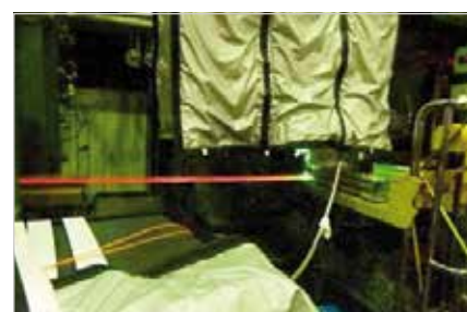
Microstructure measurement with a laser ultrasonic sensor
