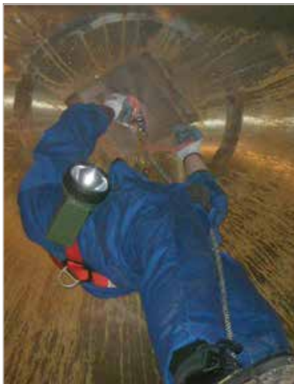
In-situ sampling of a corroded tank
