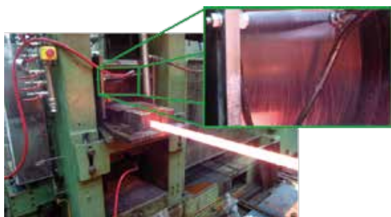
Rolling trial with recycled lubricant
