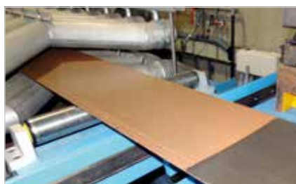
Continuous deposit of an iron oxide protective layer
