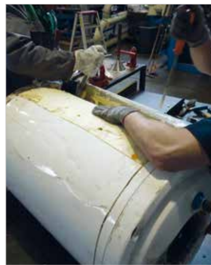
Selective dismantling of boiler
