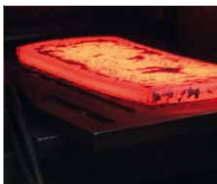
Hot rolling of multilayer material
