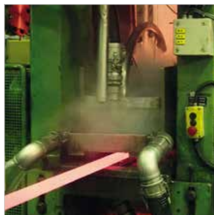
Hot rolling trials with PCD
