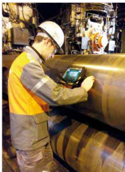
The "tablet" technology for work roll inspection
