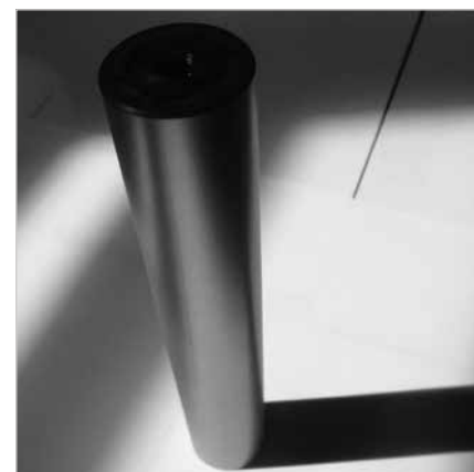
Demonstration bar coated with a Ni-P-SiC cermet
