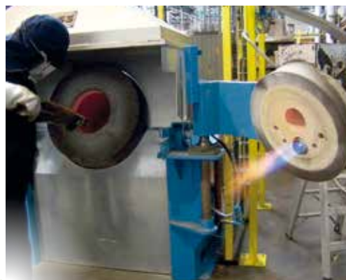
Aluminium melting unit with post-combustion
