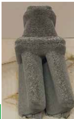
Double turbine blade ceramic mould produced by additive method
