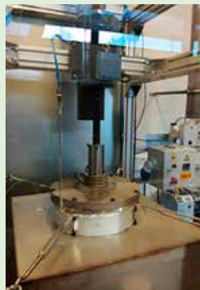
Simulation of a new bearing concept in galvanizing
