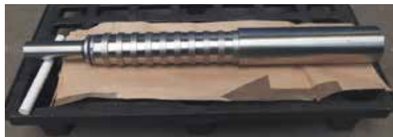
Shaft with ring-shaped samples for lab-scale rolling trials.
