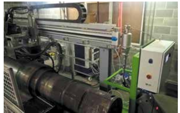
Laser cladding with powder refiller
