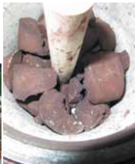
Sludge briquettes after deoiling treatment
