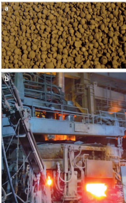
EAF plant operating with DRI – a) DRI before charging – b) Melting process
