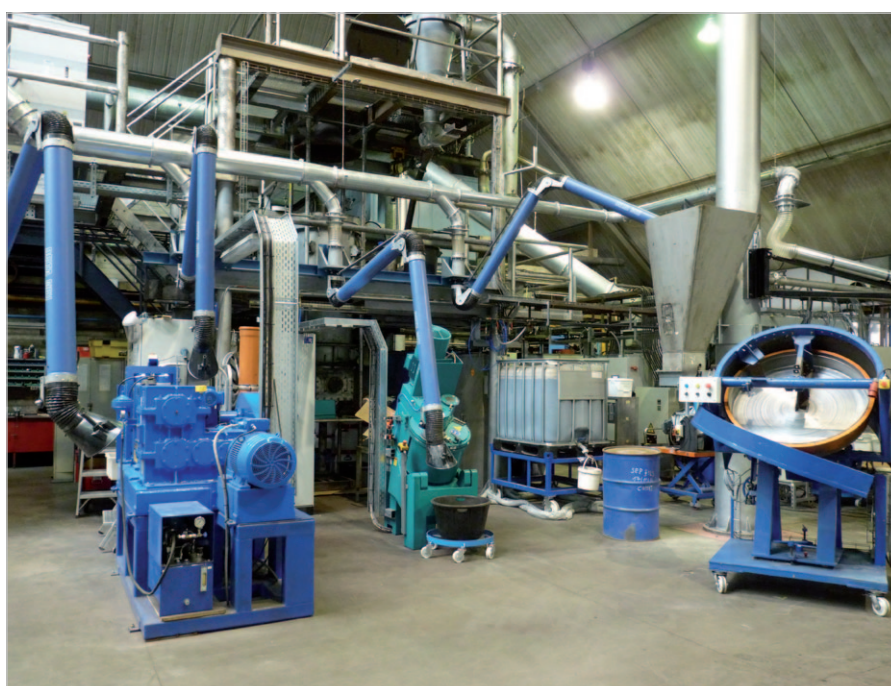
Preconditioning units available at CRM: Briquetting, intensive mixer, pelletizer
