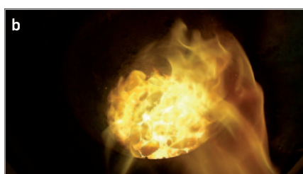
Melting of self-reducing briquettes (a: charging, b: melting)
