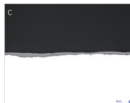
Scale after shot blasting and rolling (20% reduction)
