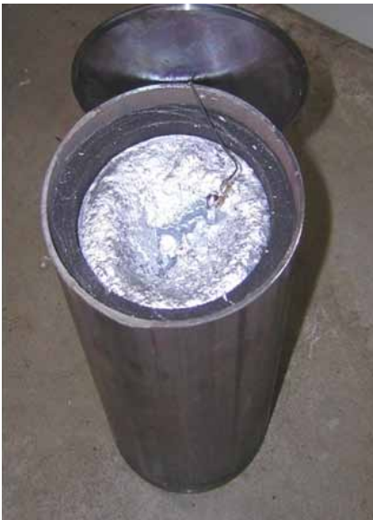
Fig. 14 Heat container for medium gas temperature filled with zinc alloy
