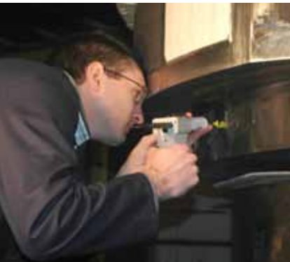
Fig. 44 Replica sampling on a massive element
