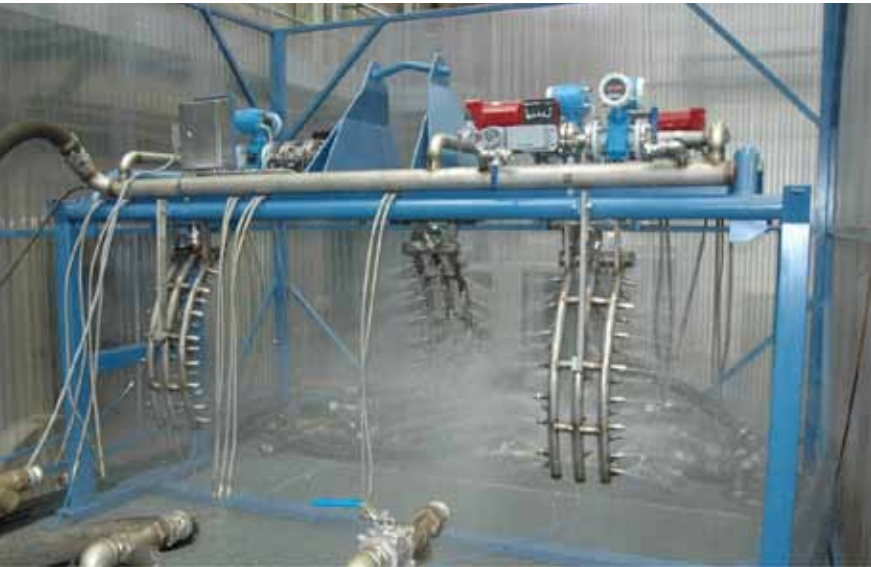
Fig. 26 Industrial prototype for the roll cooling in a sheet pile mill
