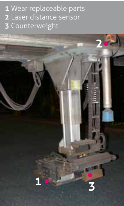
Fig. 2 Supermagnag sensor at ArcelorMittal Ghent
