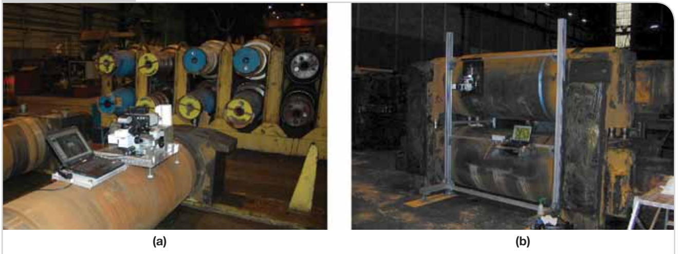
On-site microscopy with a portable microscope: (a) microscope on the roll and (b) microscope fixed vertically.
