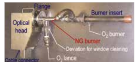
Burner equipped with the SERaFin sensor
