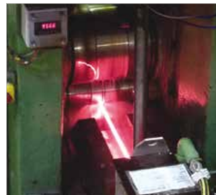
Continuous rod rolling with cermet sleeve material
