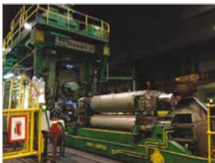
Industrial trial with alternative roll material at Tata Steel
