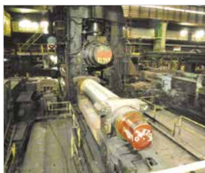
The roughing mill stand at Industeel
