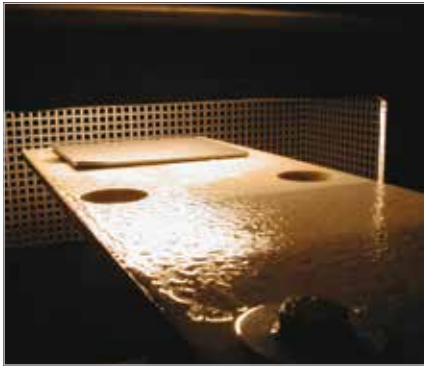
Preheating the sheet before lubrication
