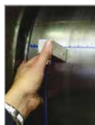
Barkhausen non-destructive stress measurement
