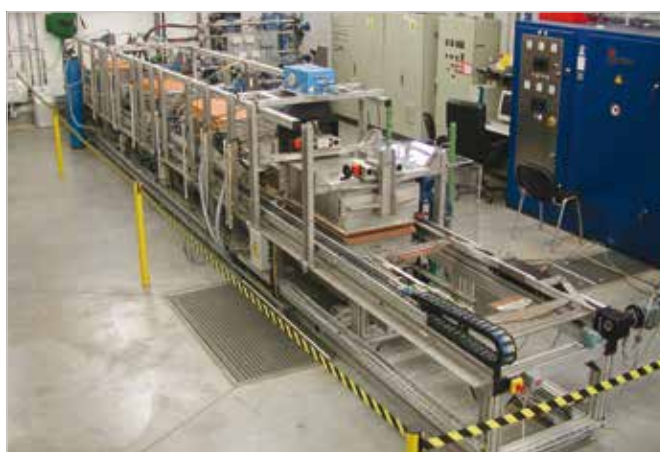
Multi device annealing (MDA) simulator
