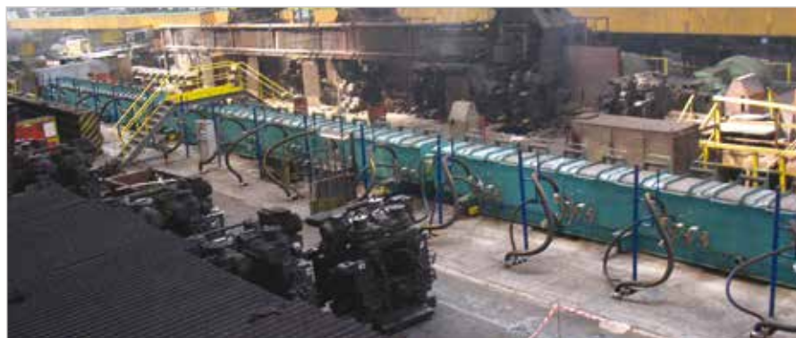
The longest “Tempcore” installation
