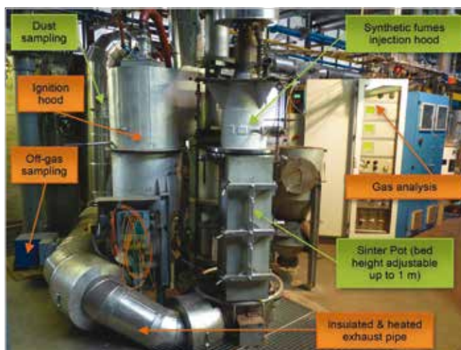
CRM Sintering pilot unit
