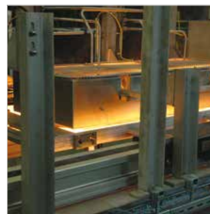
Multi device annealing (MDA) simulator
