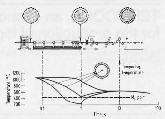
Figure 3. Schematic representation of the Tempcore process
