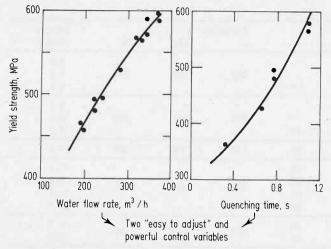
Figure 5. On line control of Tempcore
