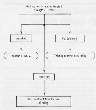
Figure 2. Methods for increasing the yield strength of rebars
