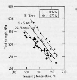
Figure 4. Example of yield strength/tempering temperature relationships
